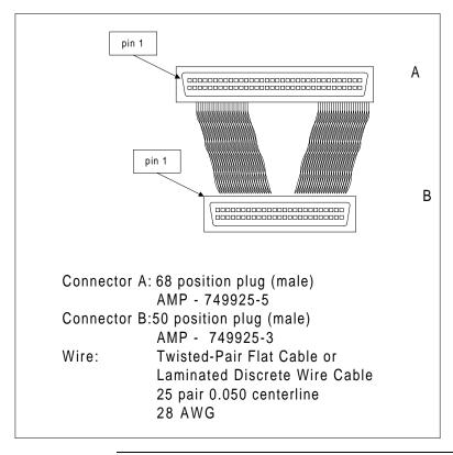
Converting from Internal Wide to Internal Non-Wide (Type 3) The cable assembly for connecting internal wide SCSI devices to internal non-wide (Type 3) SCSI devices is shown below:
